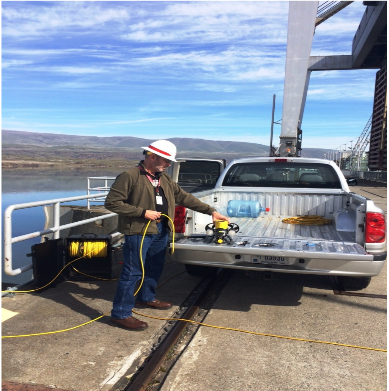
ROV inspection of MU4, MU15 trash racks 3/10; trashracks clean except for a few sticks.
